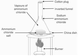
**Procedure :** Take the mixture of common salt and ammonium chloride in a china dish. Place this china dish on a tripod stand and cover it with a perforated asbestos sheet. Place an inverted funnel on the perforated sheet. Plug the opening of the funnel with a cotton
